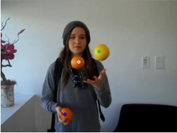
Fig. 3. Balls in the image are marked with observed positions based on k-means clustering.
